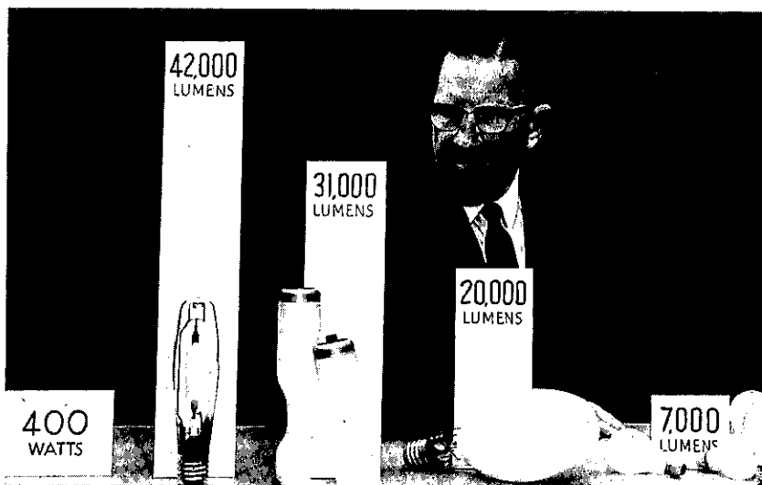
Efficiency of the new Lucalox® lamp is dramatized by Thomas M. Wallace, general manager of the Large Lamp Department. The relative light output (lumens) is shown for four types of light sources using 400w of electrical power: (l. to r.) a single Lucalox® lamp, two 96-inch-long Power Groove fluorescent lamps, a mercury discharge lamp, and four standard 100-w household lamps.
