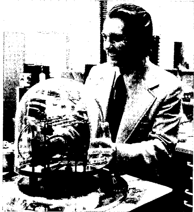
A bell jar in which Ivar Giaever performed his key experiments is shown in photo above and in diagram at left. At bottom of drawing, sketches A and B show how thin films were laid down, inside the evacuated bell jar, on glass slides.
